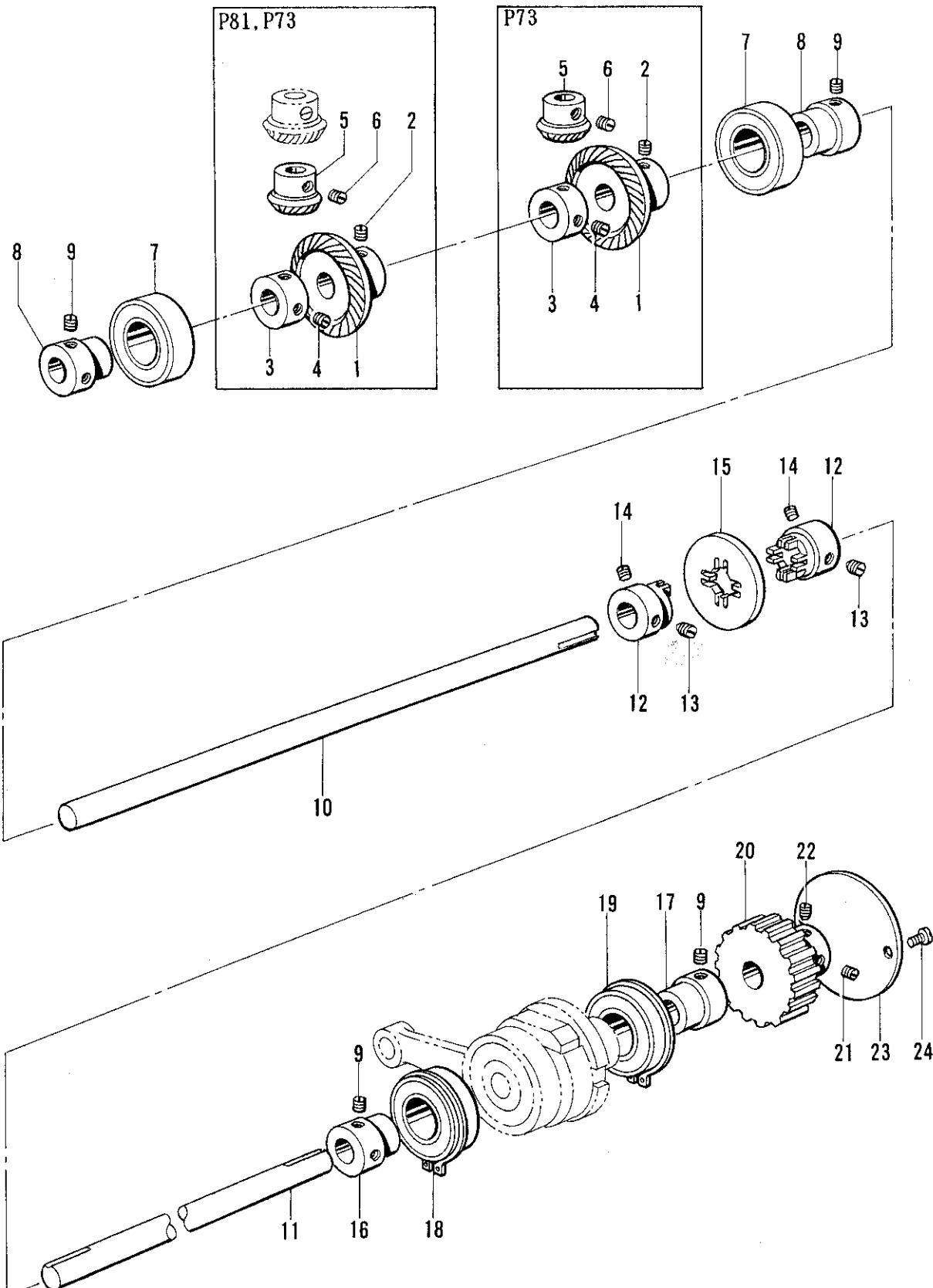
H. 下軸関係/Lower shaft mechanism/Untere Welle/
