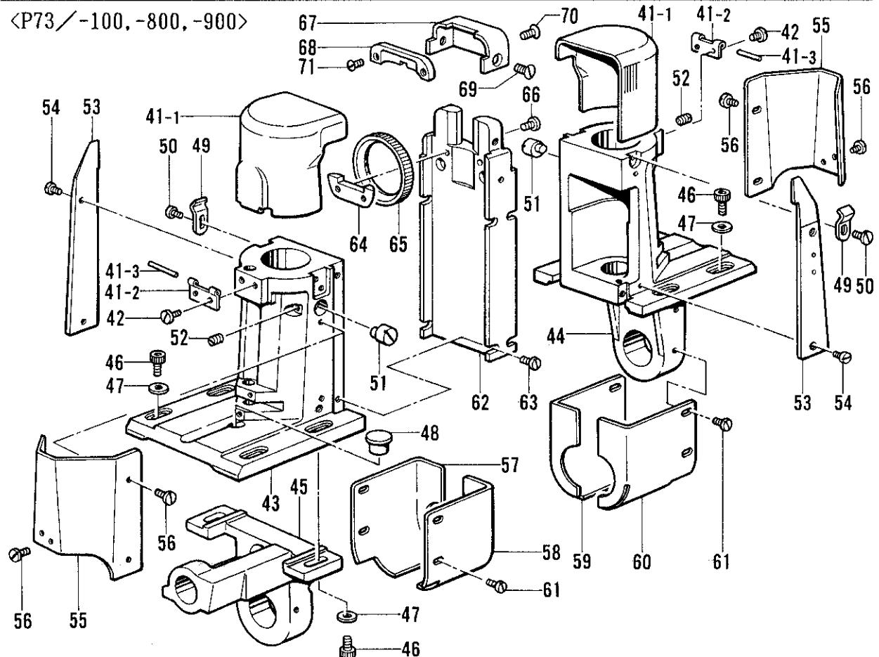
J5. カマ関係/Rotary hook mechanism/Greifervorrichtung/
