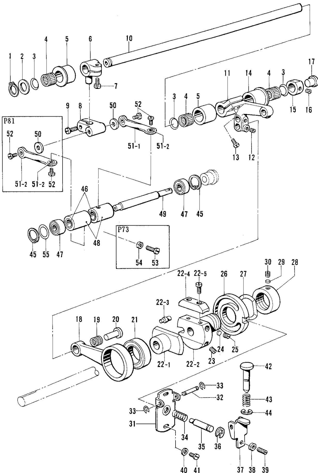
D. 送り関係/Feed mechanism/Transportvorrichtung/
