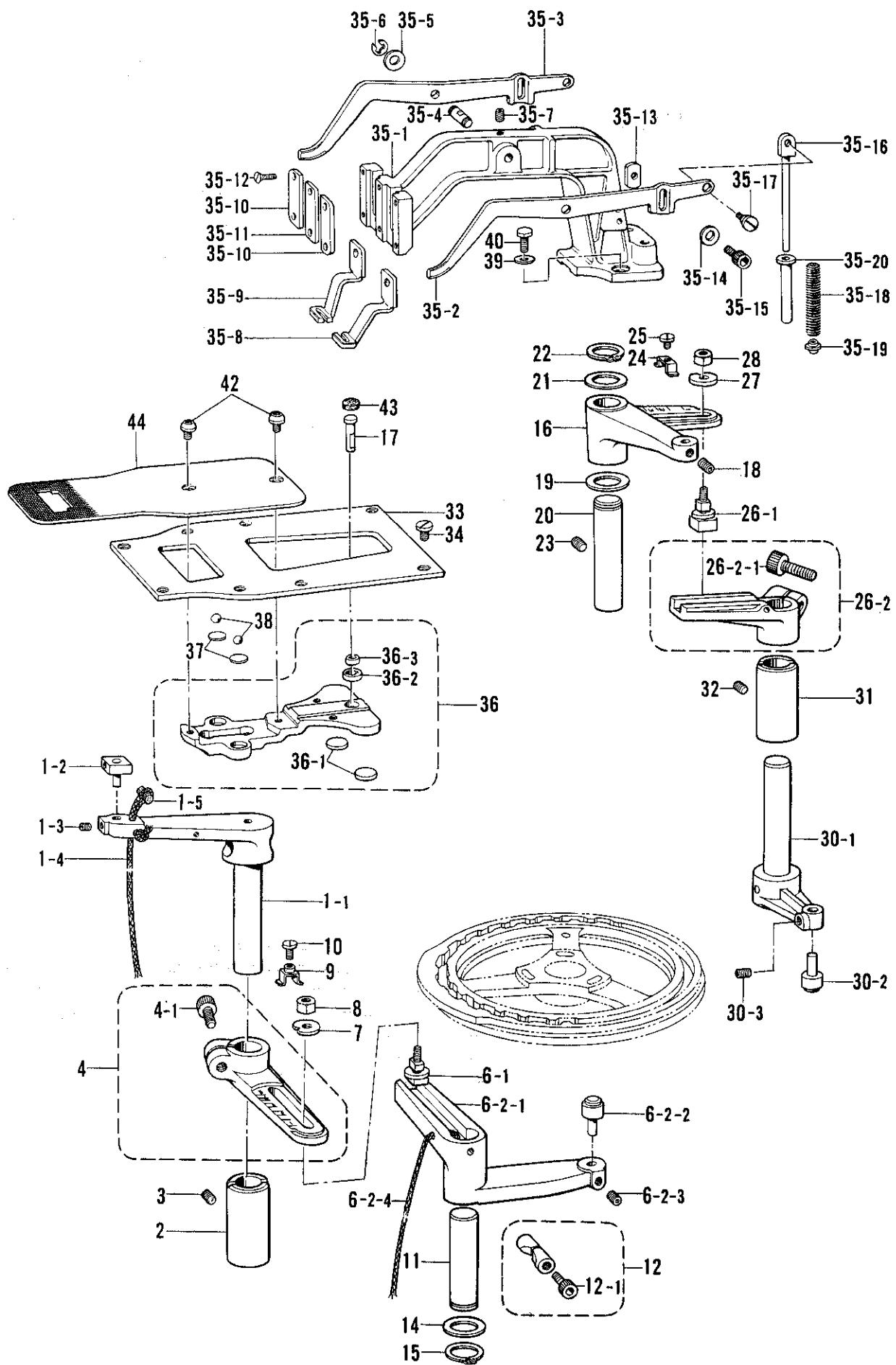
F. 送り関係/Feed mechanism/Transportvorrichtung/
