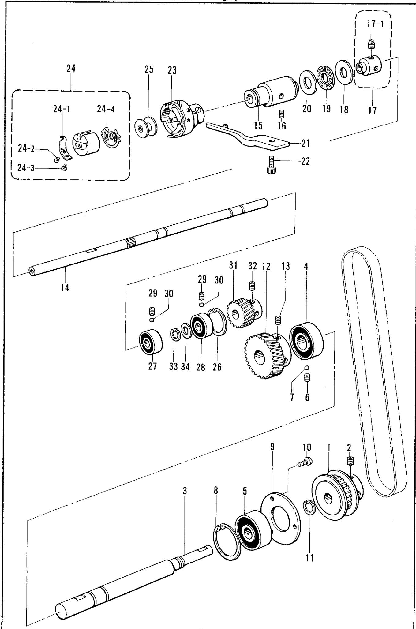
F. カマ関係/Rotary hook mechanism/Greifervorrichtung/
