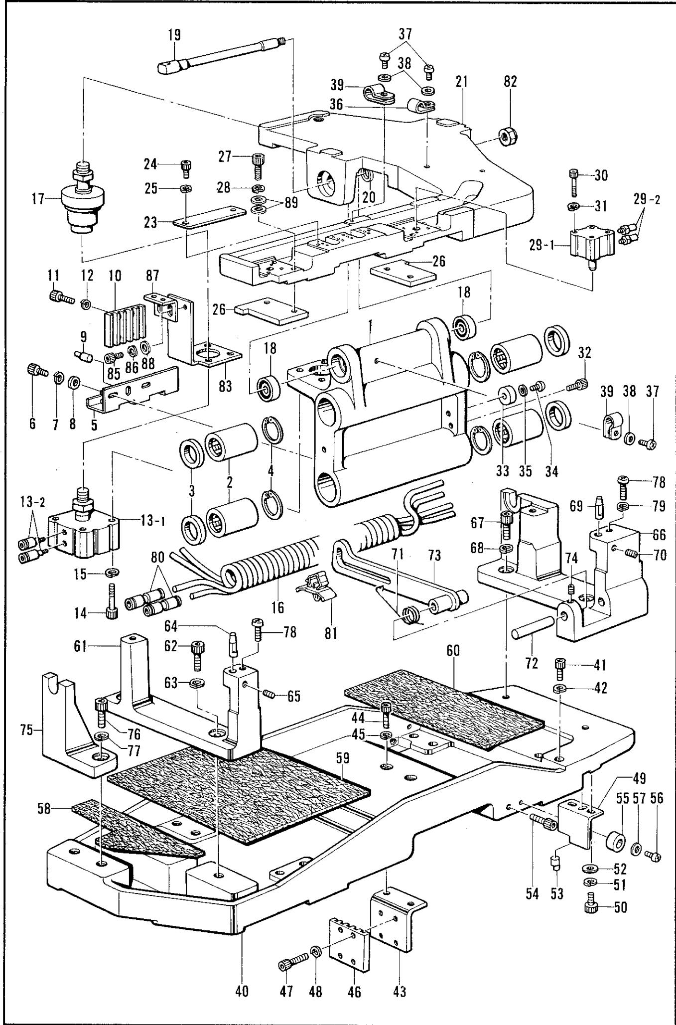
R. 駆動側・送り関係 / Drive, feed mechanism / Transportvorrichtung /
