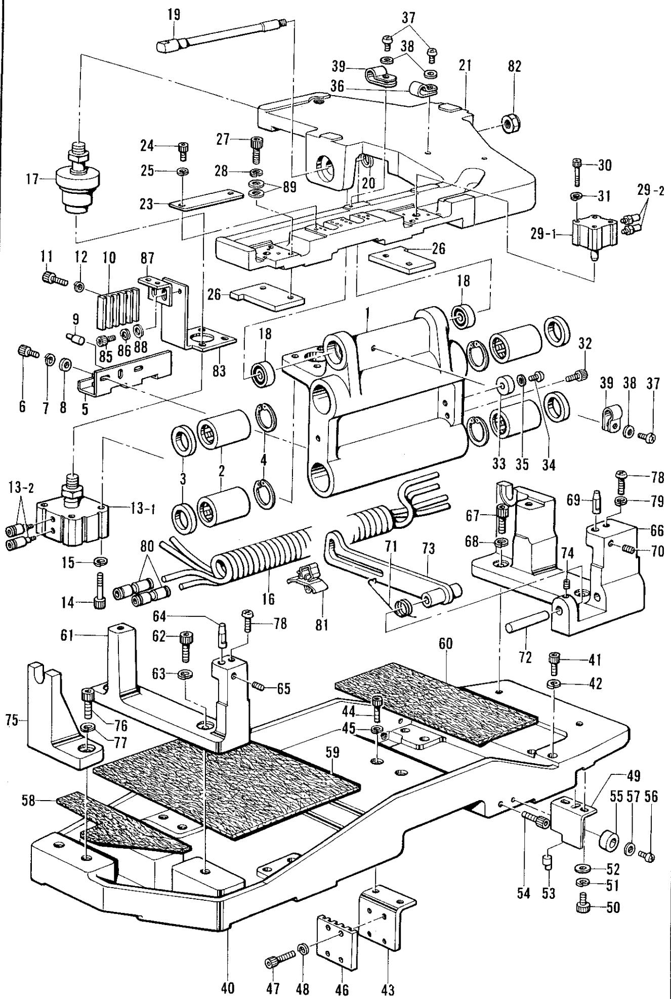
R. 駆動側・送り関係/Drive, feed mechanism/Transporvorrichtung/
