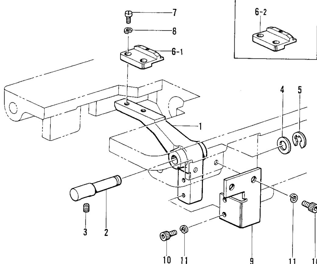
D. 糸切れ感知関係 / Thread breakage detector mechanism / Fadenbruchfühler /
